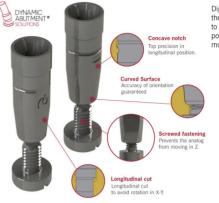
Digital analog of the dental implant to simulate implant position in a milled model.
