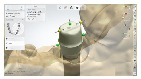
Finally, proceed to the design of the angled screw channel. Click on "Angle Screw Hole" box must be ticked.
