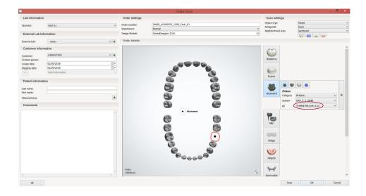
After selecting the type of work, when designing the structure the channel can be modified from  $0^{\circ}$  to  $45^{\circ}$ .
