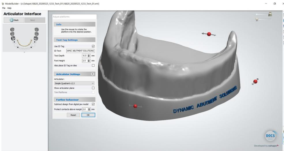
At last, the final design is obtained with the hole for the subsequent placement of the digital analog.
