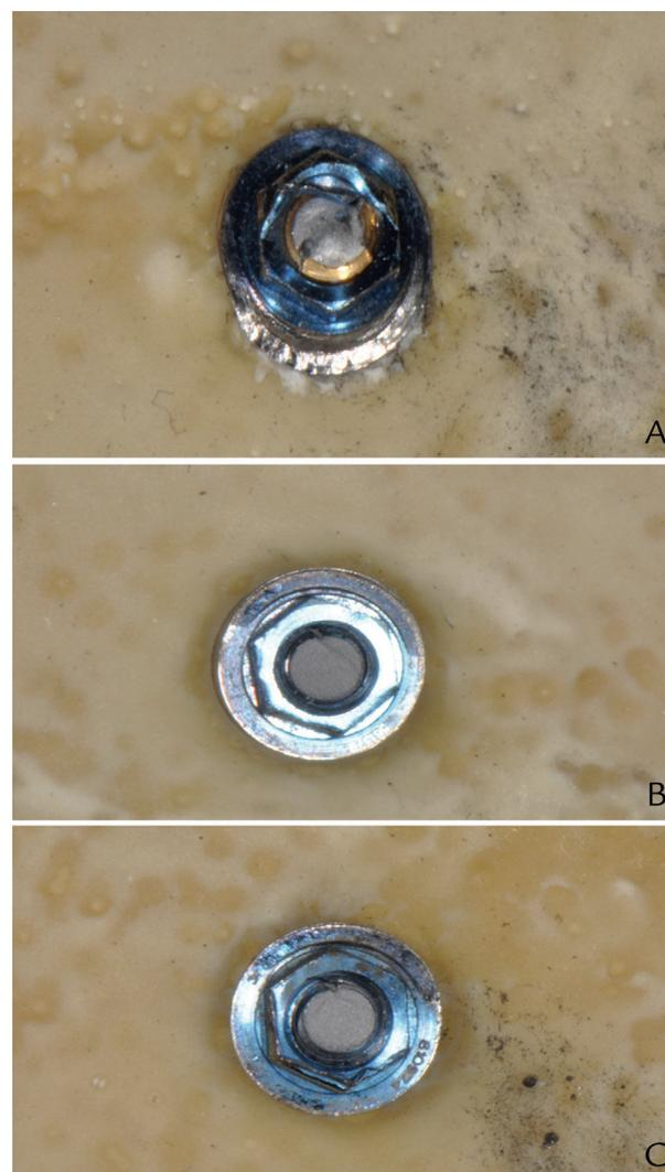
**Figure 5.** Representative screw fracture patterns after testing. A, 0-degree gold screw fracture with damage to implant platform. B, 0-degree dynamic abutment screw fracture without damage to implant platform. C, 20-degree dynamic abutment screw fracture with minimal damage to implant platform.
