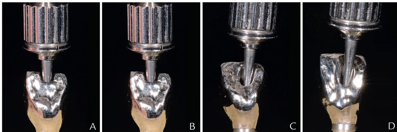
**Figure 4.** Cast specimens. A, 0-degree gold screw. B, 0-degree dynamic abutment screw. C, 20-degree dynamic abutment screw. D, 28-degree dynamic abutment screw.
