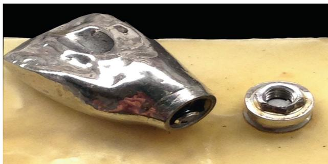
**Figure 6.** Representative specimen after fracture of dynamic abutment screw at a 28-degree angulation. Note intact platform of implant.
