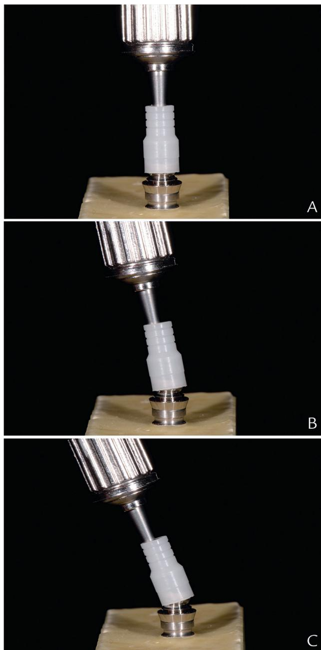
**Figure 2.** Model with castable dynamic abutment. A, 0-degree angulation. B, 20-degree angulation. C, 28-degree angulation.
