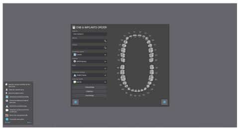
Select "Abutments" on the prosthesis family, the material and desired colour. On "Prosthesis subtype" select a work over implants to work with titanium bases. On "Implants Kits" select "DAS" and the desired code, and choose between "NR" (non-rotatory) and "R" (rotatory).
