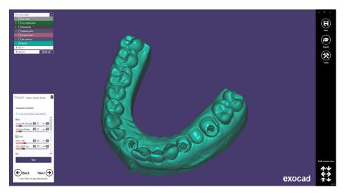
Finally, we can see the model from different views, the hole for the digital analog and the hole with the virtual analog placed.
