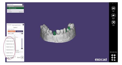
After selecting the type of work, select if the work is with straight (0°) channel or angulated channel up to 25° or 30°.
