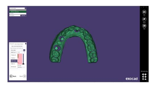
After selecting the type of work to be performed, proceed to select if you want to work with straight screw channel (0  $^{\circ}$ ) or angled channel (up to 45  $^{\circ}$ ).
