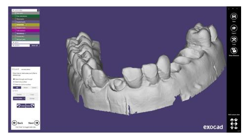
In this case proceed to close the holes and click on Next. The following Exocad screen will start with the design of the 3D model with the digital analogs and leave the space for later use of the analog.
