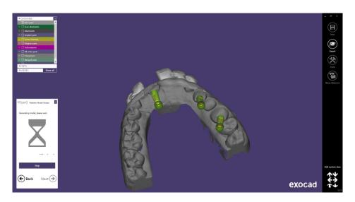
The following image shows the model with the holes. In this step you can make different modifications of the 3D, such as "Wall thickness", "Cavity fill diameter", etc.
