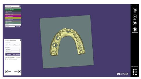
On the next screen you can modify the model, like cutting parts that are not used, "Close Holes", divide the model, etc.
