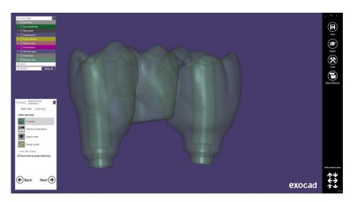
Once the work is completed, the model can be designed for subsequent 3D printing.
