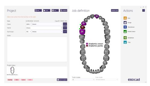
On this screen, client, patient, technician, type of work, materials, etc. is defined. The work is completely defined without specifying the brand and implant model.
