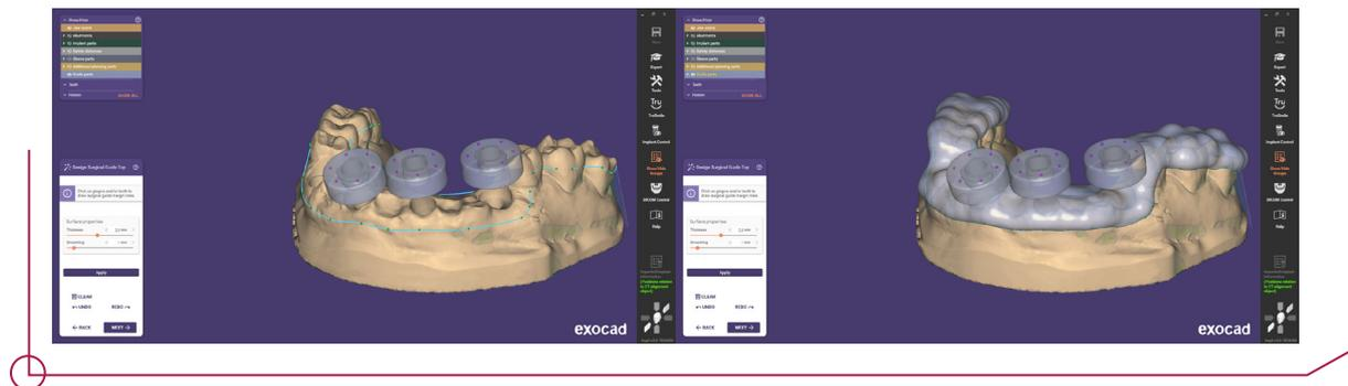
After designing the guide, adjustments can be made to it, such as holes to check that it is properly mounted, brackets to reinforce the sleeve area or adding text to the guide.
