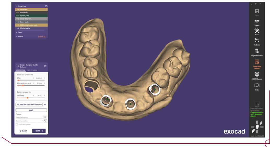
To design the upper part, draw the margin line from dot to dot where you want the guide to be placed and click 'Apply'. You can use the scroll bars to adjust thickness and smoothing.
