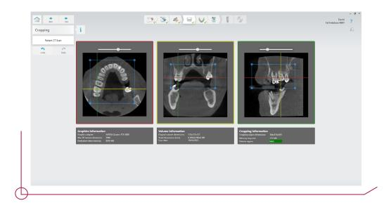
After cropping the CBCT, the panoramic curve must be set up. First, modify the position of the plane with respect to the 3D scene to adjust the cross-section where you want to have the panoramic curve. If needed, the curve can be modified manually in the axial view by using the yellow crop handles.
