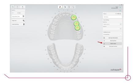
When this option is selected, the software prompts you to import the files. In the upper left-hand corner of the pop-up window, the file to be imported is displayed at all times. It is mandatory to import the upper jaw (or the lower one, depending on the jaw involved in the planning process) and the patient's CBCT (the cone-beam computed tomography systems).
